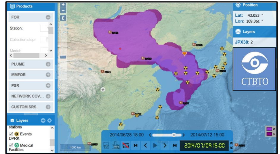
3-day multi-model field of regard for JPX38 for collection for sample ID 2862643 using Web-Grape
