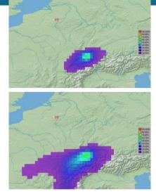
Examples of the Network Coverage for DEX33 in winter 2020. **Upper Panel:** Xe-135; **Bottom Panel:** Xe133. The red sign indicates IPF in Fleurus (IRE). The color-coded percentage indicates the area monitored by DEX33 with sufficient sensitivity to trigger detection.
