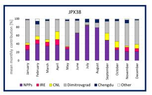
Mean monthly contribution of Xe-133 emissions from individual sources as observed at IMS stations. The results are based on operationally produced ATM results (backward modelling) using meteorological data from ECMWF.
