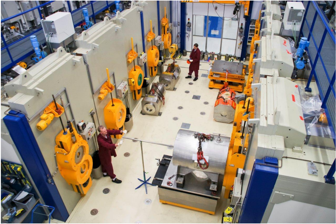
Back Side of Petten Mo-99 Hotcells
