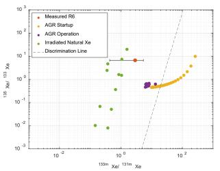
Calculation of the radioxenon isotope ratios shows values right of the nuclear explosion discrimination line during AGR start-up and left during routine AGR operation.
