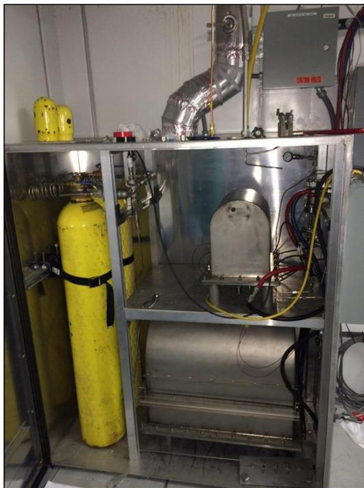
**Figure 4.3.** Argonne National Laboratory Off-gas Recovery System for Mini-SHINE Experiment. Pumps for the system are enclosed in vessels to prevent leaking.
