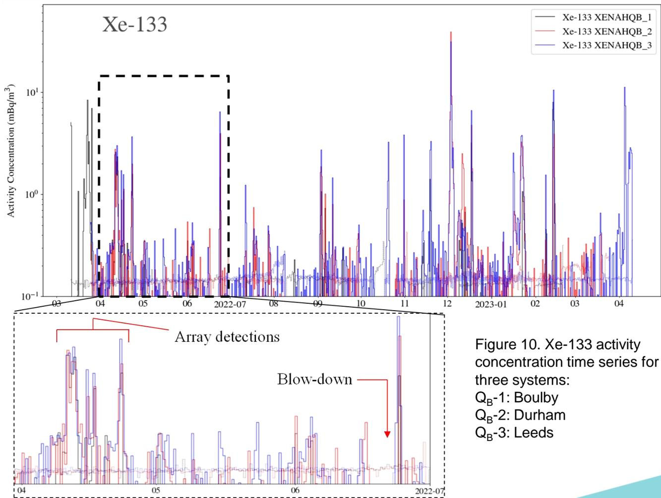
Figure 10. Xe-133 activity concentration time series for all three systems:
