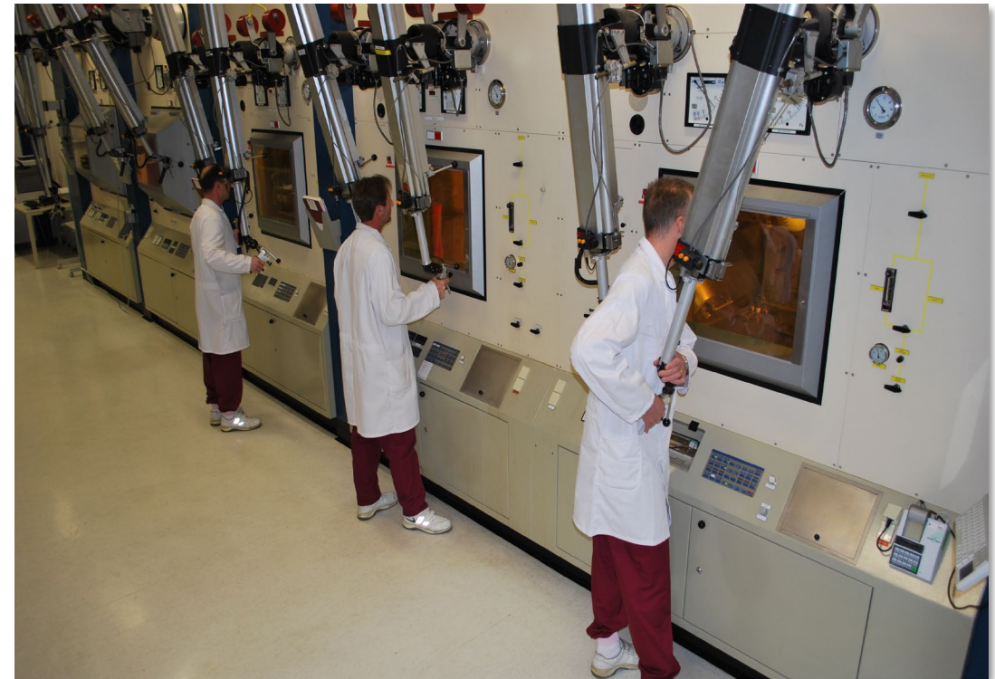
One of Curium's Mo-99 Production lines in Petten
