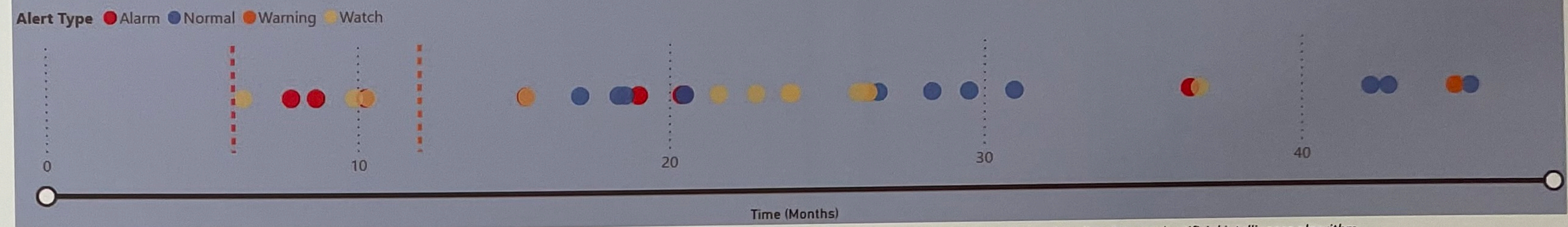
Figure 6 – The output of the analysis algorithms, which predicts the time until servicing is required for each detector using live data, factory baseline data, and artificial intelligence algorithm.
