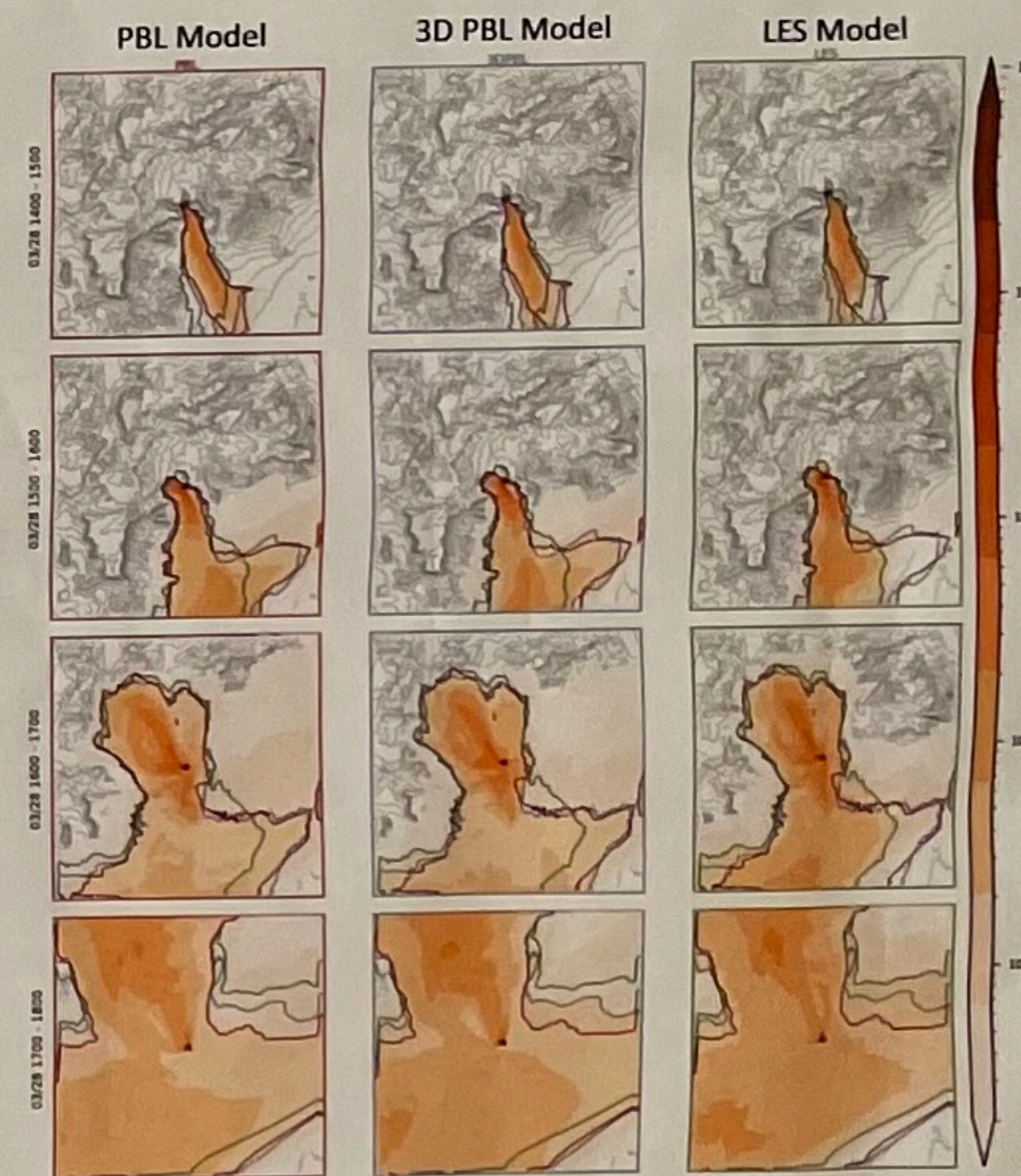
Birds eye comparison of predicted plumes using three methods to parameterize turbulence and mixing
