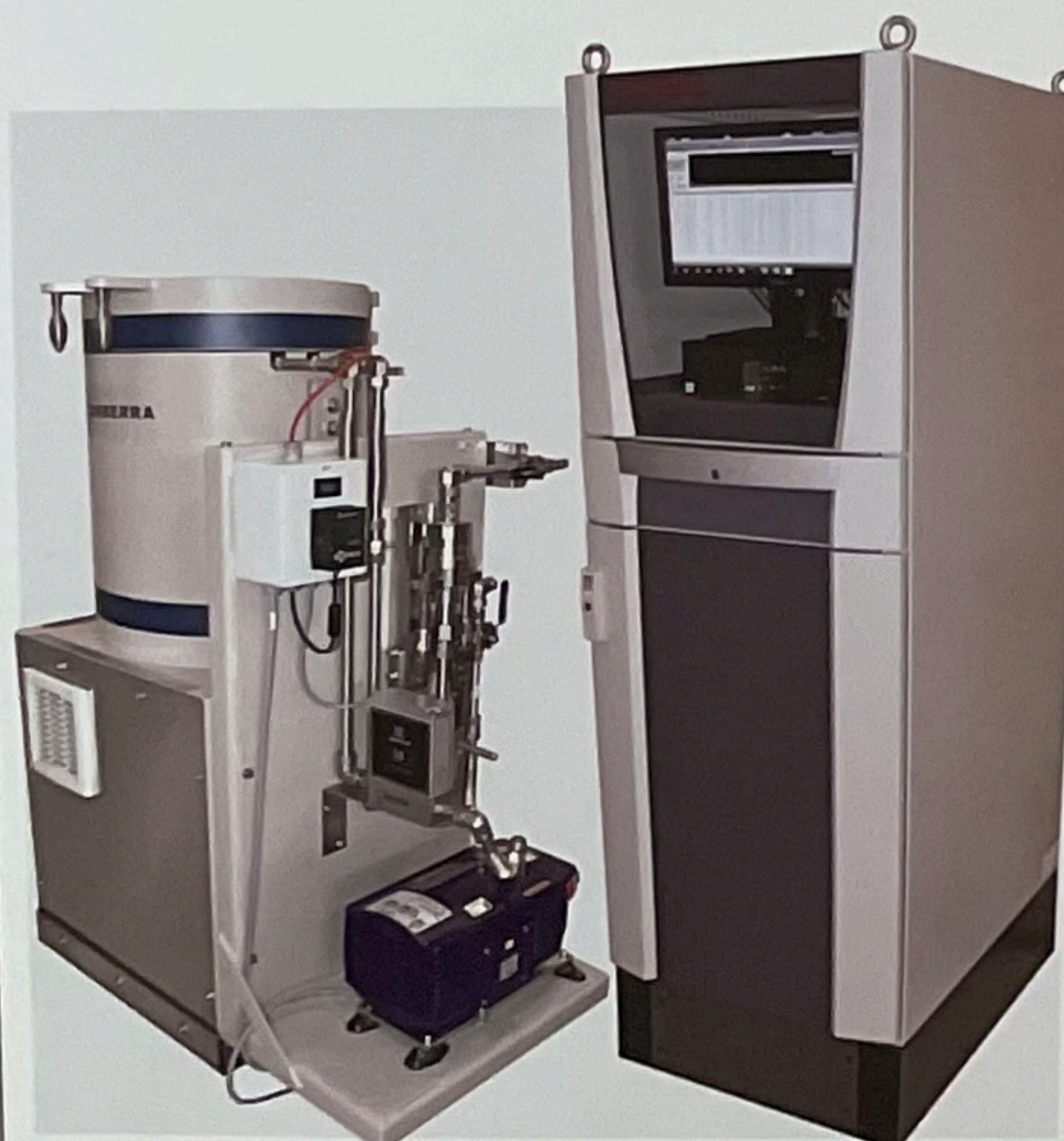
Figure 1 – The Mirion Spectroscopic Stack Monitor System with the sampling skid (left) and control cabinet (right).
